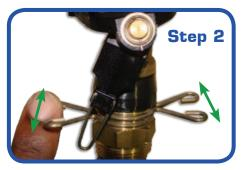
Step 2) The adjustable stop clips may be moved around to any position on the sprinkler base to facilitate part circle operation. One stop clip will be the right side stop for the reverse trip lever to engage and the other stop clip will be the left side stop for the reverse trip lever to engage. The sprinkler will then operate back and forth between the stop clips in the desired pattern set by the adjustable stop clips.
