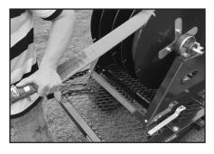
4) Pull the hose in a straight path away from the hose reel until the entire hose has been deployed.
