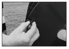
2) Unhook the bungee strap from slot on the divider and remove from the hose end.
