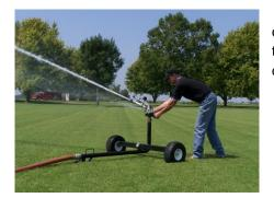
5) Pressurize and test the sprinkler. Refer to the sprinkler manufacturer's optimal pressure range for the nozzle that is installed. When functioning properly, the sprinkler performance will match the manufacturer's performance chart for distance under acceptable wind and atmospheric conditions.
