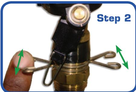
**Step 2)** The adjustable stop clips may be moved around to any position on the sprinkler base to facilitate part circle operation. One stop clip will be the right side stop for the reverse trip lever to engage and the other stop clip will be the left side stop for the reverse trip lever to engage. The sprinkler will then operate back and forth between the stop clips in the desired pattern set by the adjustable stop clips.
