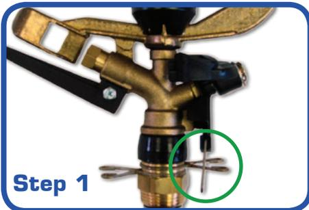
**Step 1)** For part circle operation, the reverse trip lever on the Koala may be flipped down in an engaged position as shown in the left image labeled *STEP 1*. This will allow the reverse trip lever to engage the adjustable sprinkler stops allowing the sprinkler head to operate in a part circle mode.
