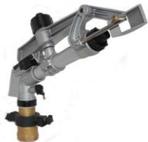
3) Examine the drive arm. The drive arm should move freely but not have excessive sloppy movement on the pivot shaft that may indicate wear in the drive arm bushing or bearings. Drive arm water deflection spoon must also be inspected for excessive wear at the water point of contact.
